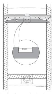
Fig. 23 Leveling the mounting bracket on the studs
